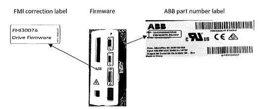
Note: The spare part packaging is labeled with the GE part number and the Microflex drive is labeled with the ABB part number.
