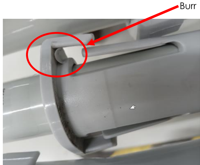
Figure 1: Siderail connector with burr
