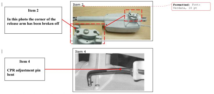
A modification to the CPR design was introduced for beds manufactured after April 2001 and a retrofit kit, part number 806.399, has been developed which allows pre-April 2001 beds to be modified in line with the later specification. The later design prevents over travel of the CPR lever and thus prevents the mechanism from being damaged.
